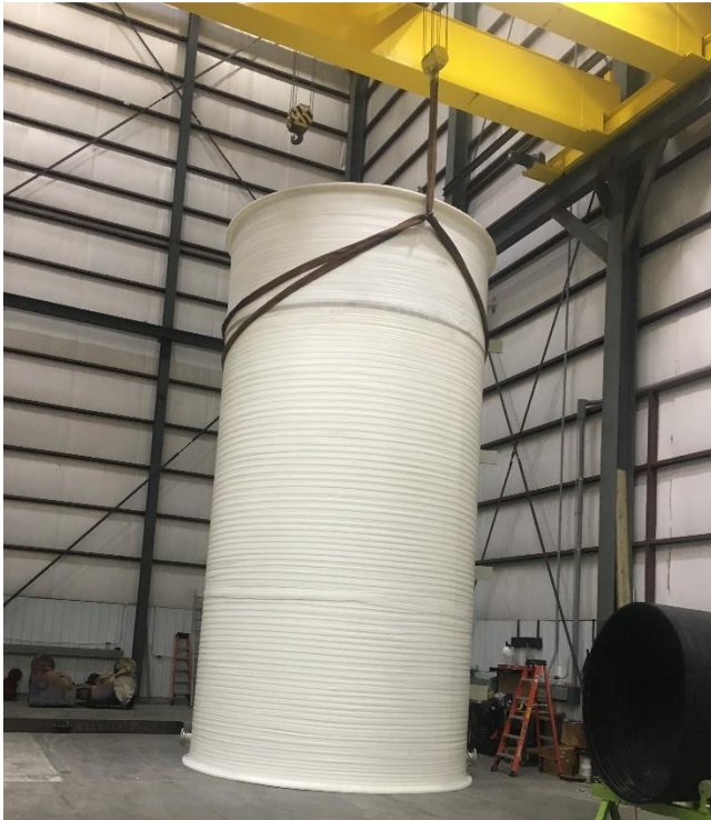
Front View of Tank while being choked
