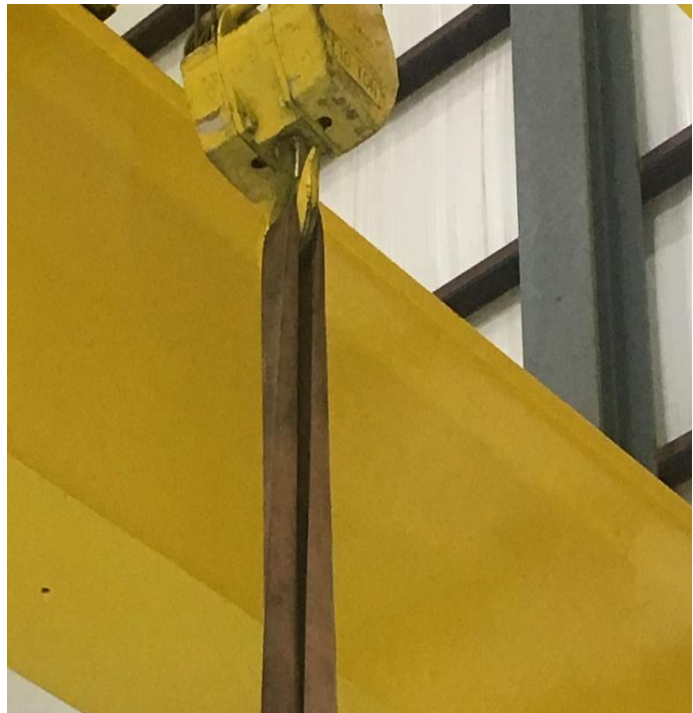
Picture 2: Endless nylon sling connected to the crane hook.
